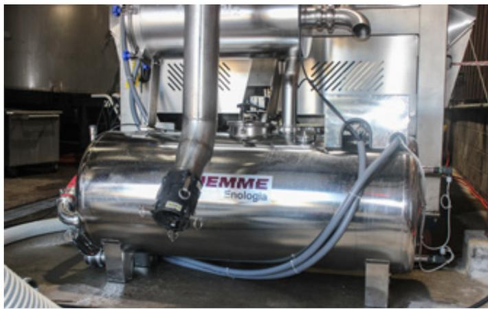
The Diemme Neutral 2 surge tank maintains the inert atmosphere in the ullage of the press pan as juice is pumped out.
